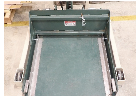
Fig. 4.4. Locked Rear Wheels of Lift Truck
