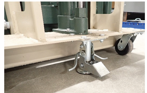
Fig. 4.4. Locked Rear Wheels of Lift Truck
